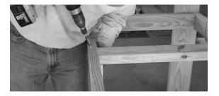
10 Attach the shelf (K) to the back legs (A), keeping bottom of shelf flush with bottom edge of top stretcher (C). Use a combination square and clamps to help keep the shelf square and level. Use glue and 3" screws through the back legs and into the shelf, and use 2" screws from the back of the top stretcher and into the shelf.
