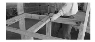
**07** Install bottom front stretcher (I) to front edge of both lower stretchers (F), keeping tops flush. Use glue and 2" screws.
