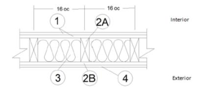
GYPSUM BOARD (Interior): Two layers USG Firecode® C Core, complying with ASTM C1396, min. 5/8 in. thick, 4 ft. wide applied vertically, fastened to framing. Face layer joints staggered with base layer and covered with paper tape and joint compound.
