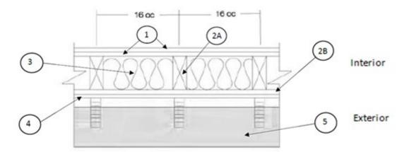
GYPSUM BOARD (Interior): Two layers Type X complying with ASTM C1396 min. 5/8 in. thick, 4 ft. wide applied vertically, fastened to framing. Face layer joints staggered with base layer and covered with paper tape and joint compound.
